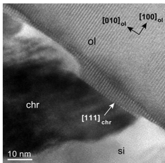
Fig. 7. HRTEM image of the contact between host olivine and a chromite lamella within an inclusion. The contact is sharp and parallel to  $(100)_{ol}$ ; the  $(010)_{ol}$  fringes continue to the boundary, but with a slight structural tilt immediately adjacent to it.
