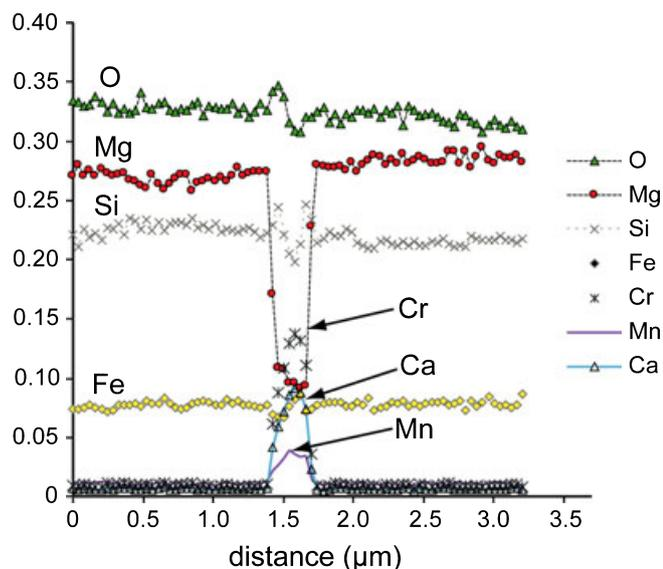
Fig. 3. Composition profiles (EDS analyses) along the line scan indicated in Fig. 2a. The vertical axis indicates fractional compositions assuming an  $M_2SiO_4$  formula.
