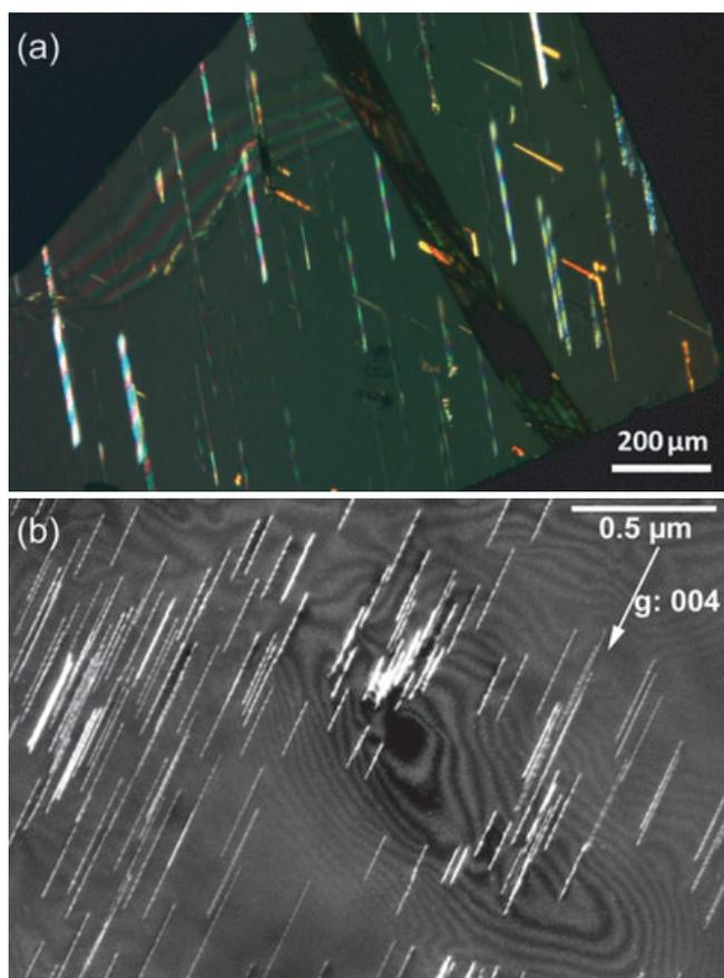
Fig. 1. a) Optical microscope image of tubular inclusions in the Fukang pallasite as seen using crossed polars. b) Weak-beam, dark-field TEM image of laboratory-generated  $[001]_{ol}$  screw dislocations in olivine produced at a pressure of 11 GPa at 1400 °C.  $g: 004$ . The figure is from Couvy et al. (2004).
