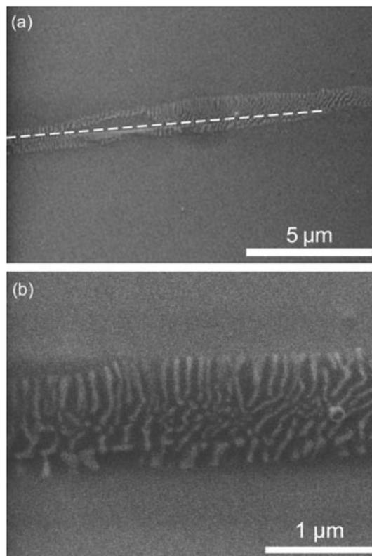
Fig. 4. SEM images of a lens-shaped tubular inclusion in olivine that is oriented to view down the inclusion long axis, which is parallel to  $[001]_{ol}$ . a) Low-magnification image depicting the cross-sectional shape of the inclusion. There is an approximate medial line running the length of the inclusion. b) Higher-magnification image showing wormy contrast produced by the chromite lamellae.
