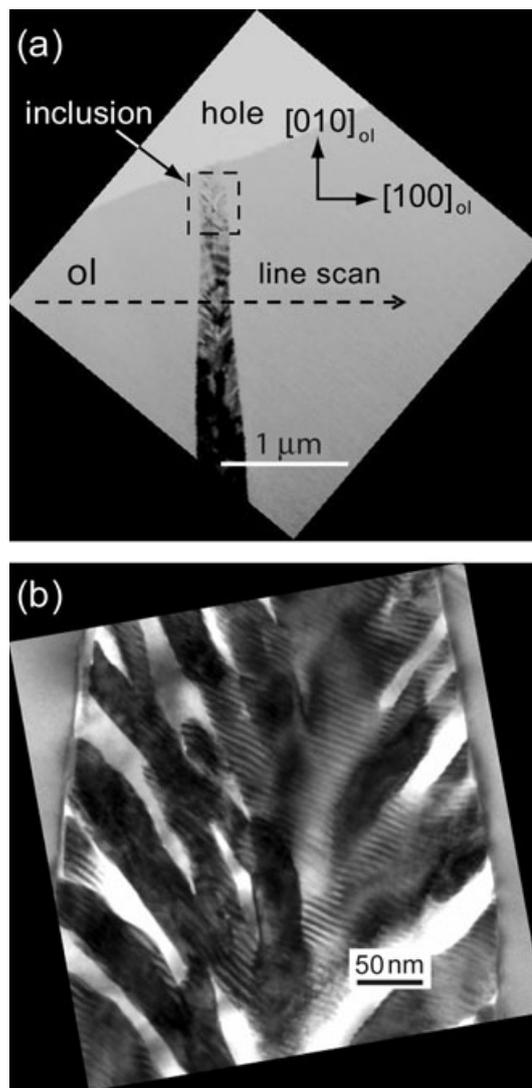
Fig. 2. a) BFTEM image of a cross section of a lens-shaped tubular inclusion within olivine (ol; darker gray) at the edge of a hole (light gray at top of figure). b) Magnified image of the boxed area in (a), optimized to enhance contrast and details of the texture within the inclusion. The regions showing dark contrast are chromite, and the white areas within the inclusion are silica.
